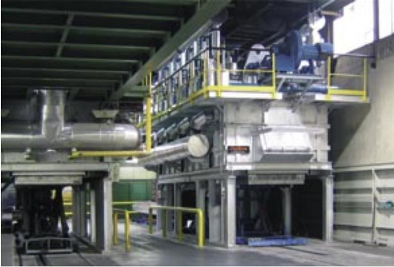
Hood furnace system · For homogenising aluminium parts
