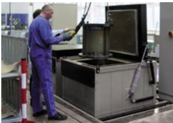
Air-circulation pit-type furnace
